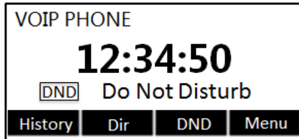
Figure 57 - DND Enabled on All Lines
