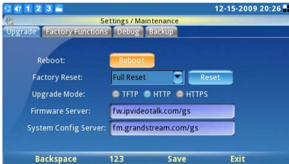
Figure 119: Factory reset the phone using the keypad
