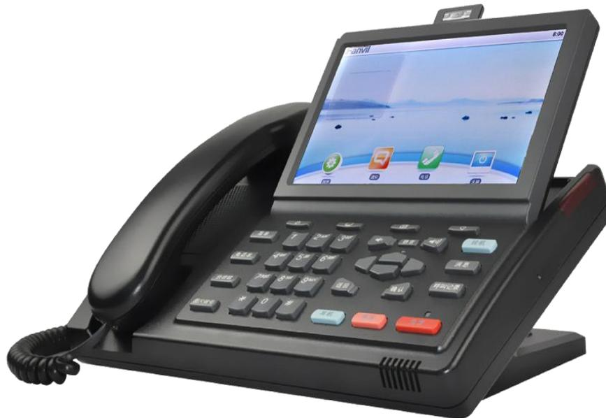
SE780 is the advanced IP video phone based on Android OS 2.1. It is equipped with the latest Broadcom video chipset, a 7" adjustable LCD touch screen with 800x480 pixels and a 2M pixel camera. Android OS guarantees the easy customization for telecom operator and service provider. The intelligent OS, superior video quality, rich applications and affordable price, ensure SE780 IP video phone is the Pioneer for next generation smart video telephony.
